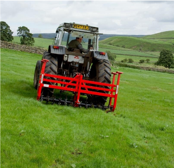
Soil aerator (near-surface equivalent to sub-soiling) – source: © Helen Keep, Yorkshire Dales National Park Authority
