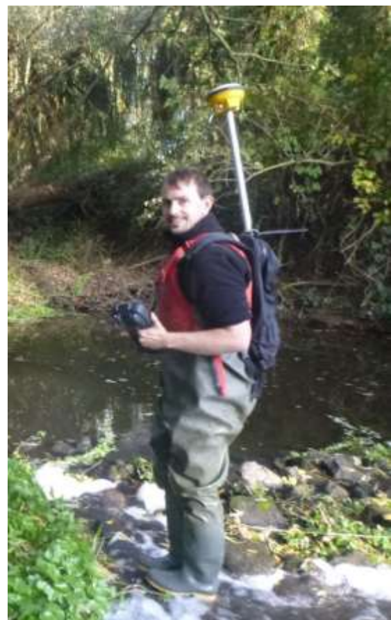
Figure 2 & 3. Sampling in areas inaccessible by boat with portable Trimble positioning equipment
