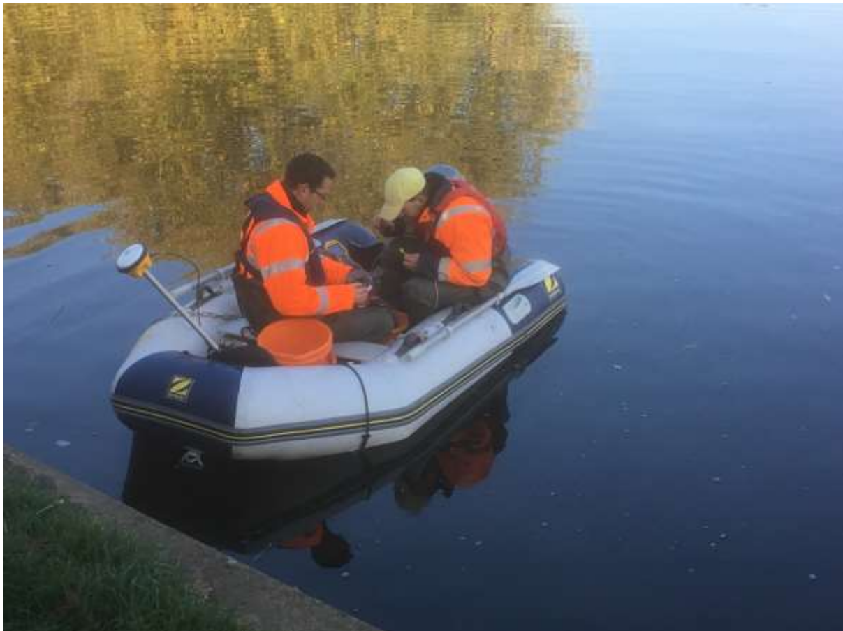
Figure 7. Image of zodiac inflatable dinghy with 6hp outboard engine, Trimble GNSS positioning system.
