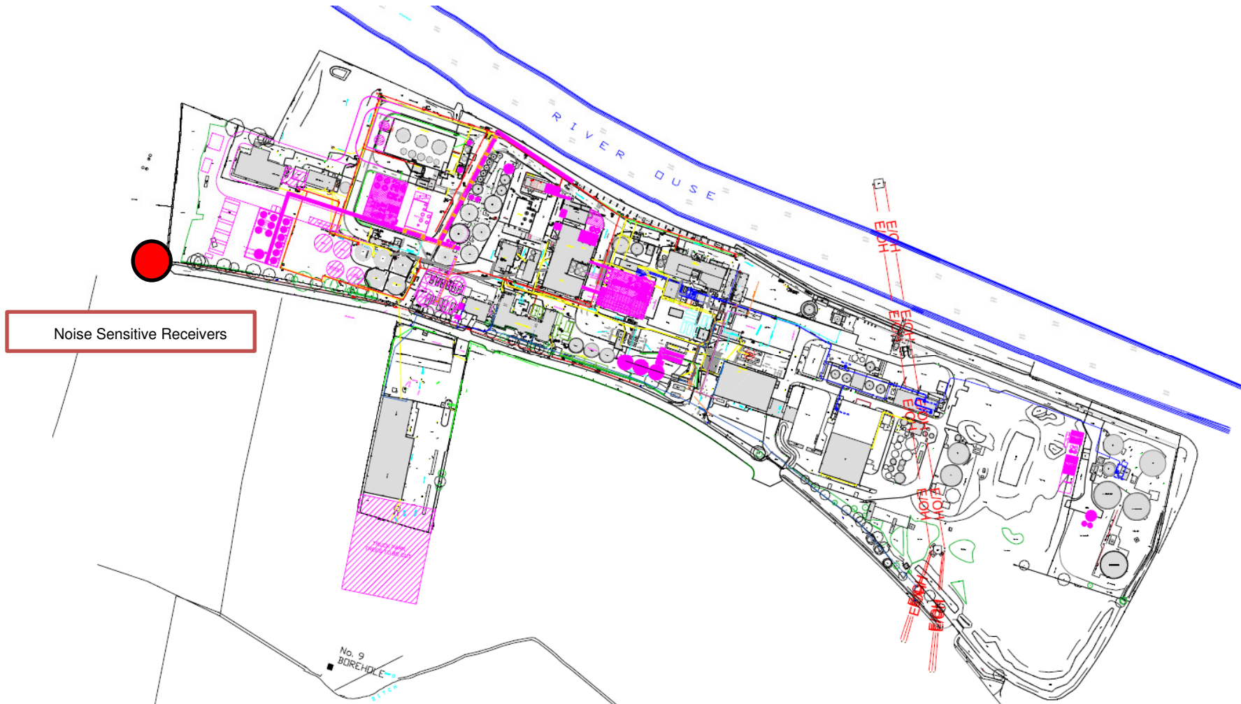
Plan view of the SEDAMYL UK Plant and foreseen new noise sources
