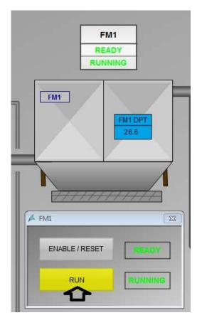
AV1 FM1 is installed to protect filter by cooling air in case of high temperature threshold, but it can also be opened to reduce water consumption to quencher Q1.
