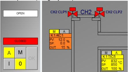
Put P1 in automatic regulation to maintain optimal set points for refining furnace
