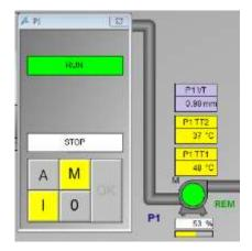
Press "M" and "OK" to confirm manual mode selected. The press "I" and "OK" to start ID fan P1 in manual at 30-40% capacity.
