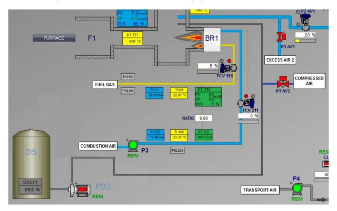
Install lance L7 in lower part of K1 then start pump PD2. Open the compress air to lance by valve K1 AV2.
