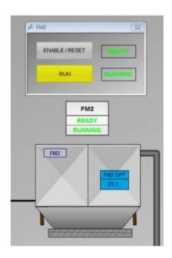
AV1 FM2 is installed to protect filter by cooling air in case of high temperature threshold. In case of high high temperature alarm refining furnace door must be closed.
