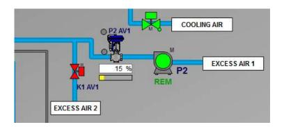
Excess air fan P2 is very important during "REDUCTION" phase to provide combustion/excess air for methane coming from refining furnace.
