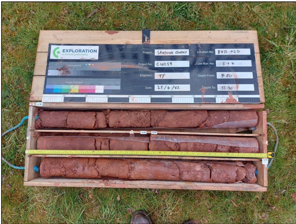
BH22-02D, core runs 3 & 4: 50.80m—55.30m bgl.
