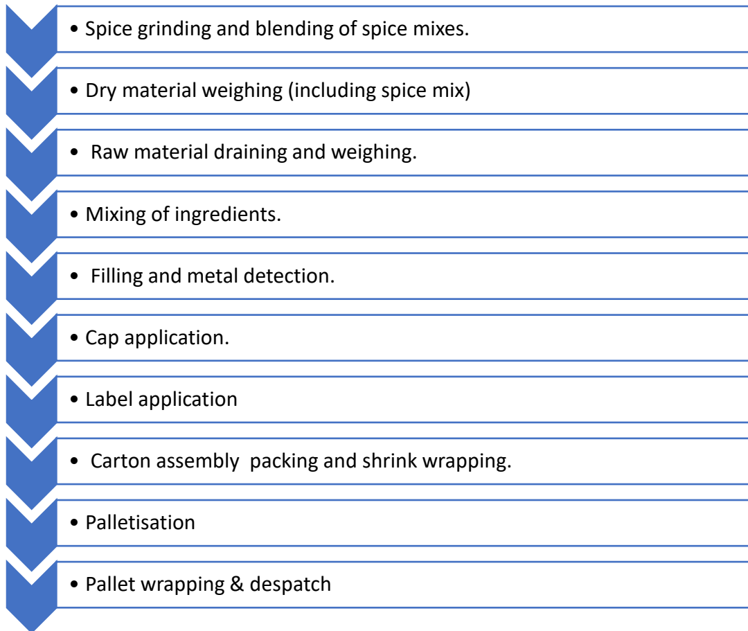
Figure 3 Process flow for paste, pickles and chutney in glass and plastic jars.
