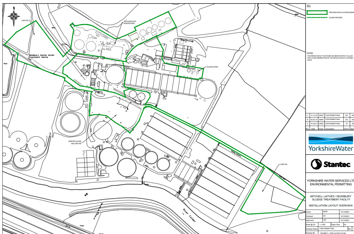
Fig 1 – Mitchell Laithes STF showing the installation boundary (green) and associated assets some of which may have the potential to cause bioaerosols
