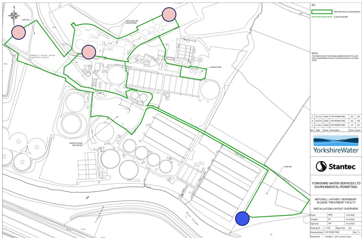
Figure 3 – Mitchell Laithes STF Site Plan showing the installation boundary (green) with bioaerosol monitoring locations marked (blue dot = upwind, pink dot = downwind)
