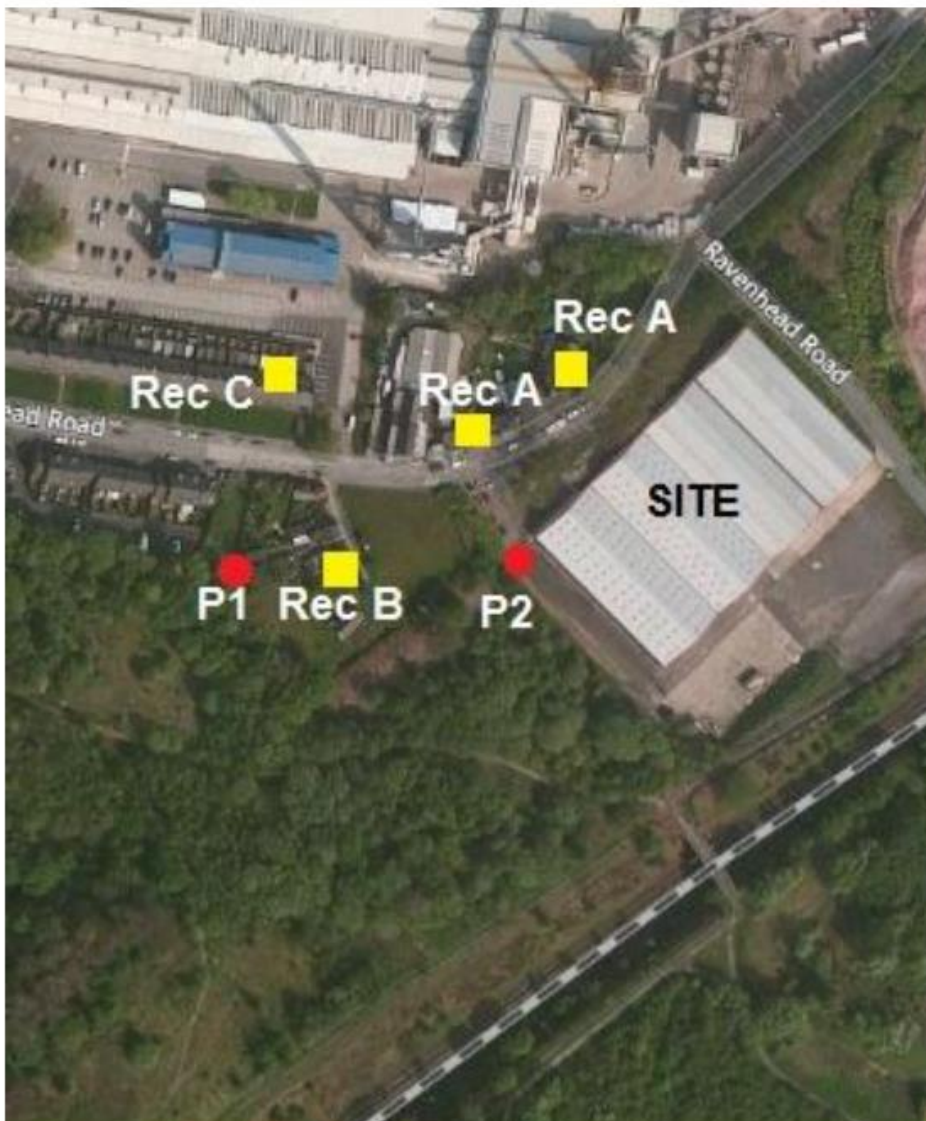
Figure 2-2 – Veolia 2016 noise impact assessment noise measurement locations
