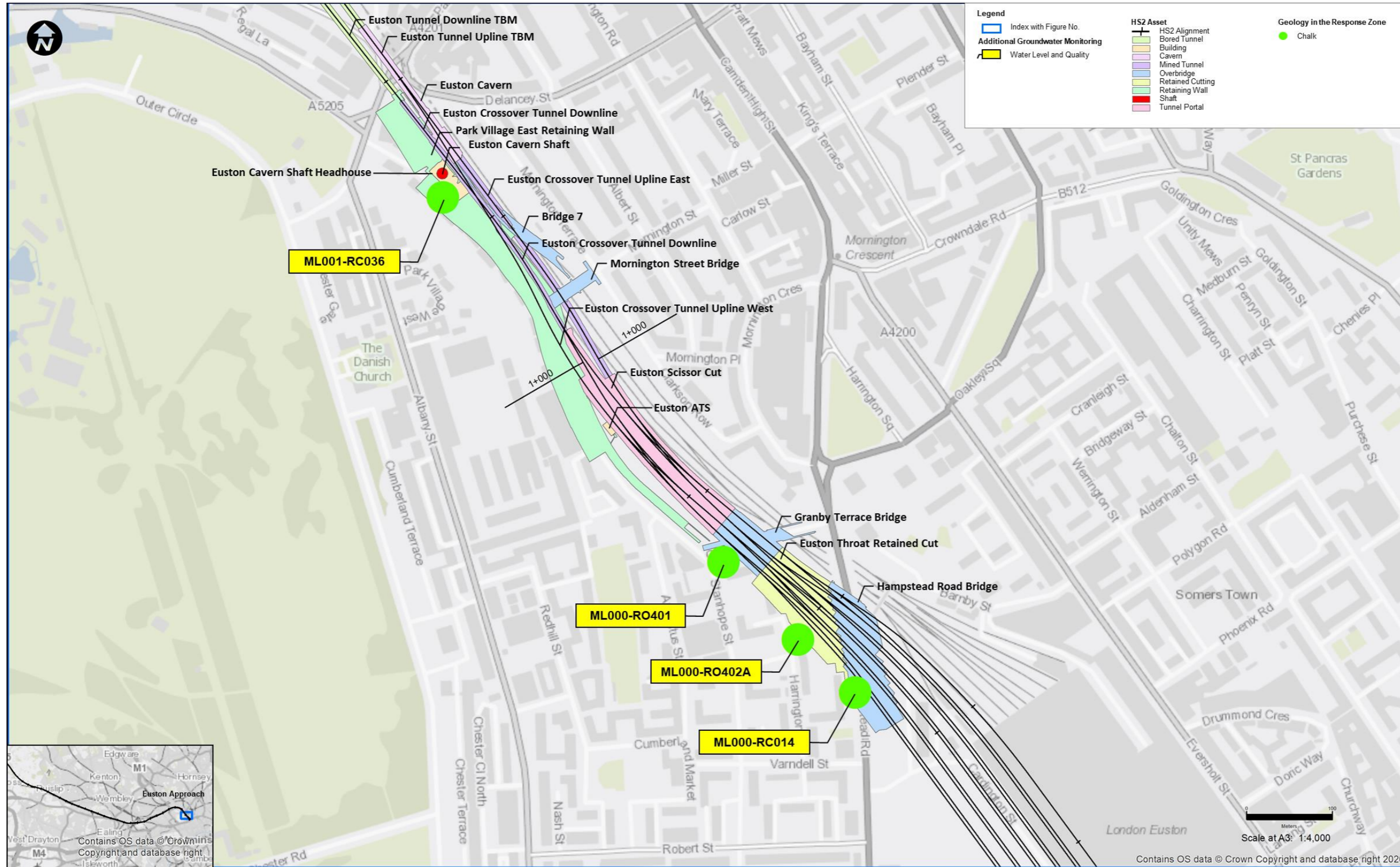
Figure 11 Groundwater Monitoring Plan - Euston Approach
