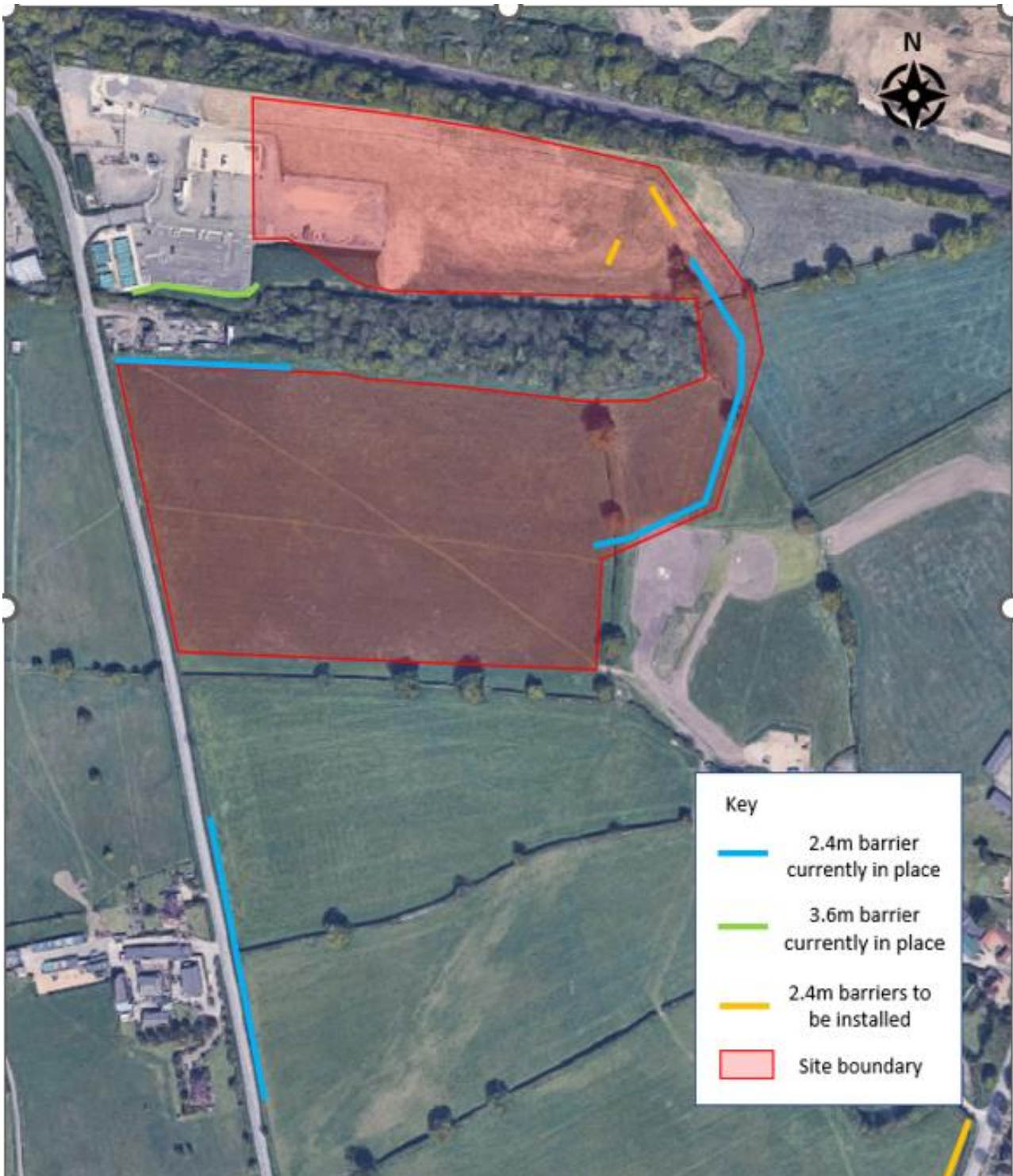
Figure 8: Implementation of noise barriers.
