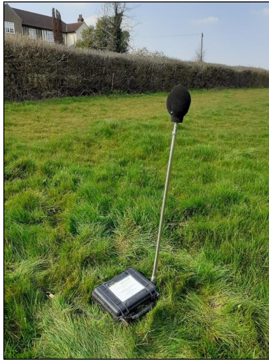
Figure 4: Noise monitoring systems setup, MP03.
