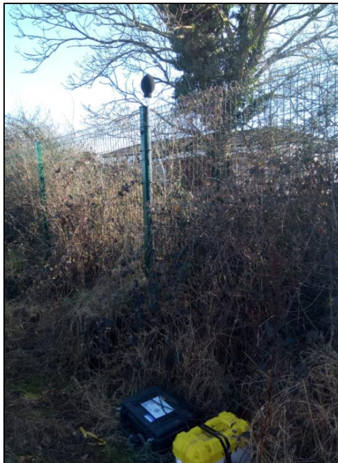
Figure 2: Noise monitoring systems setup, MP01.
