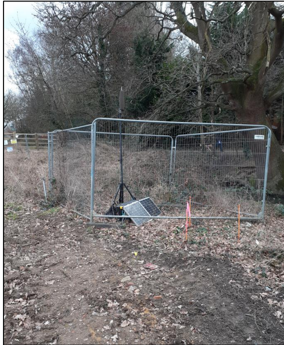
Figure 6: Noise monitoring systems setup, MP05.
