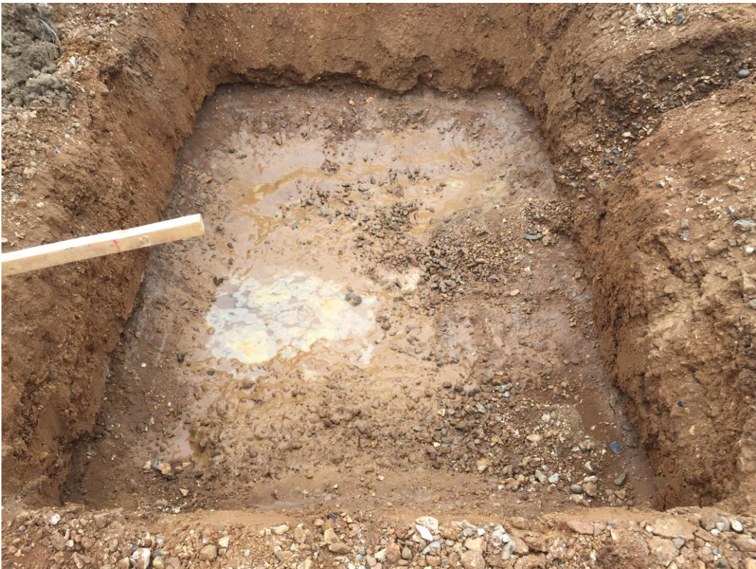
Photograph No. 4: Trial Pit 2 (31 st May 2019) – trail pit at end of test.
