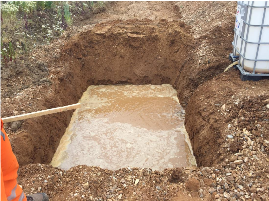
Photograph No. 3: Trial Pit 2 (31 st May 2019) – filling trial pit with water. Pit dug by backhoe.
