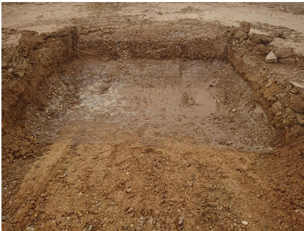
Photograph No. 2: Trial Pit 1 (2 nd May 2019) - trial pit at end of test.
