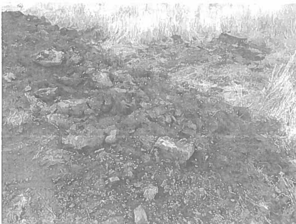
Photograph 12. Backfilled trial pit, more clay evident with refractory bricks and some slag
