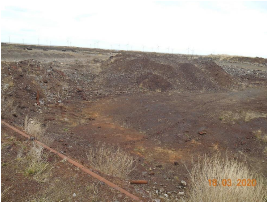
Plate 8 - View looking north showing typical spoil heaps of iron slag waste material.
