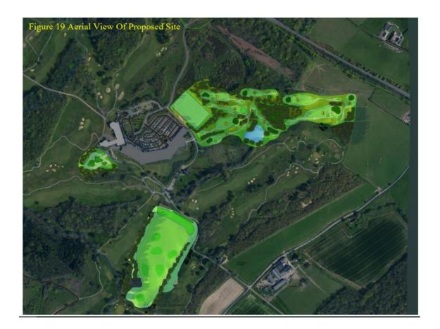
Whilst the area is relatively large, the recontouring is limited in depth. On average the contours will increase 1.0 to 1.5m, with some localised thicker layers to accommodate new tree planting. The placement of materials in the 3 areas is discontinuous in places. As can be seen in the cross sections of the largest area to the east below, with the darker green representing the additional material.
