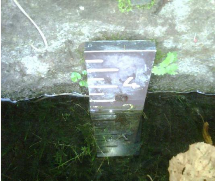
Figure 3 : Level gauge in the Canal on 26/11/21 (reading 2.25 inches)
