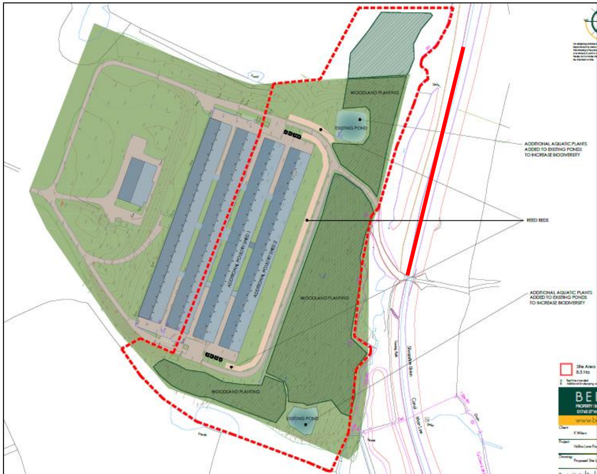
Figure 8. Proposed mitigation plan (red line indicates 125 m length of LWS where critical load is exceeded)
