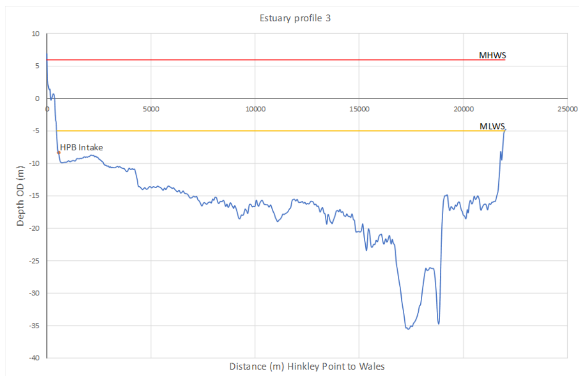
Figure 1 Location of HPB intakes. The figure shows from left to right a northerly transect from HPB through the HPB intake caisson to close to the Welsh coast. The depths of mean low water springs (MLWS) and mean high water springs (MHWS) are also shown.
