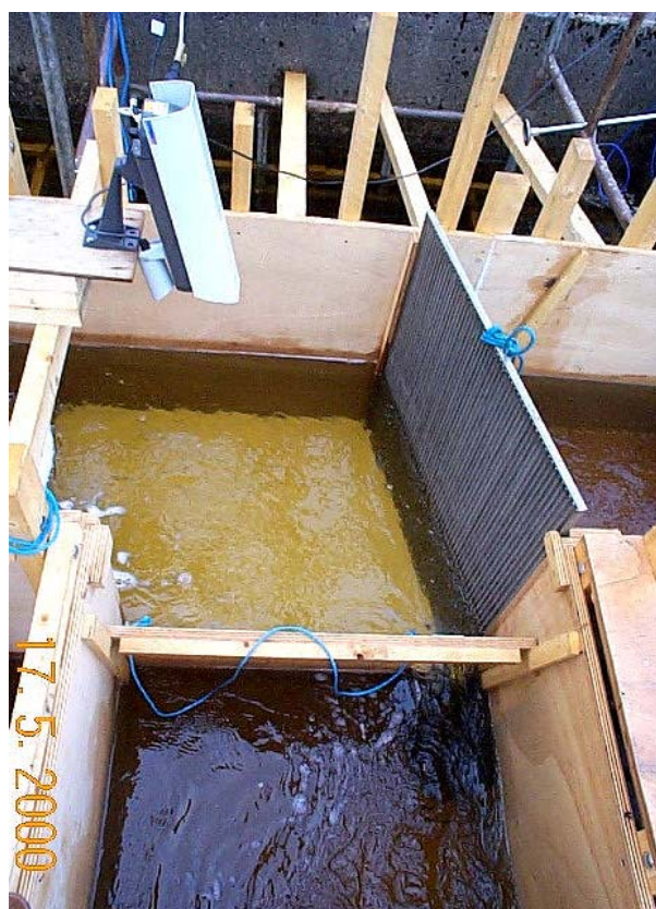
Plate 3.3 Experimental apparatus used in bar rack trials at Gaur (Clough et al. 2000).
