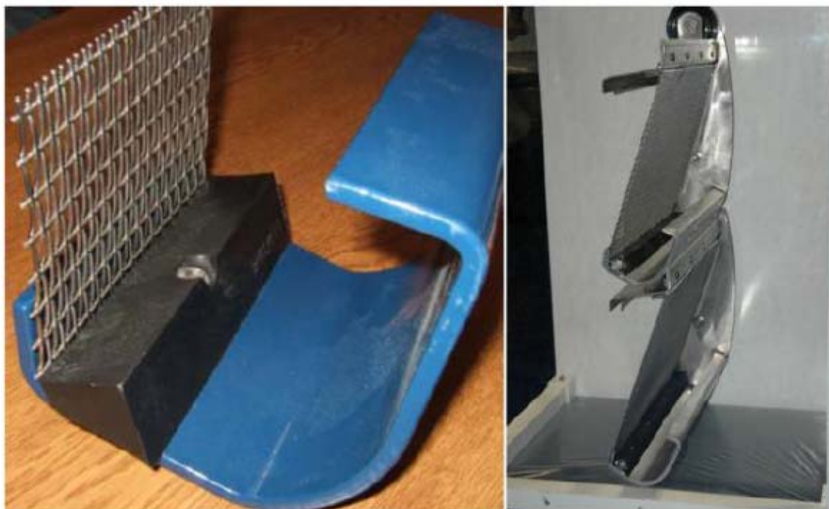
Figure 5.5 Anticipated fish recovery bucket design
