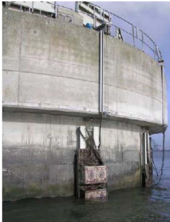
Figure 4.4 Diagram showing the SP mounting units at Doel and the remote retrieval mechanism
