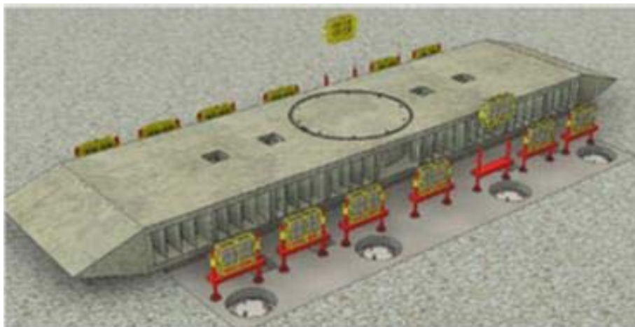
Figure 5.15 Depiction of SPs mounted on discrete subsea structures supported by posts cast into the intake head foundation chamber.
