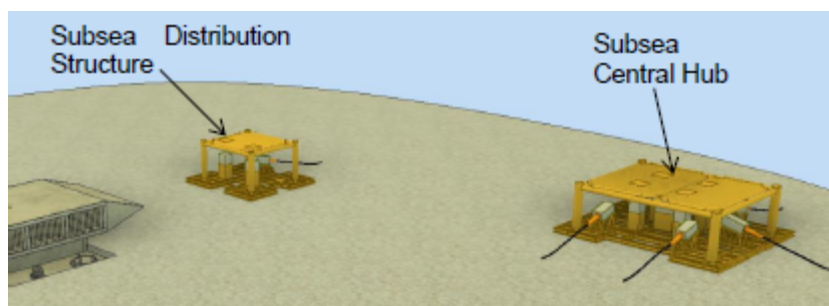
Figure 5.20 Depiction of a subsea central hub with underwater transformer
