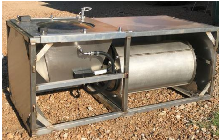
Plate 1 –MkIV 30-600 Sound Projector with APCS fitted for deployment at Barkley Lock, USA (access side panel removed for photograph)
