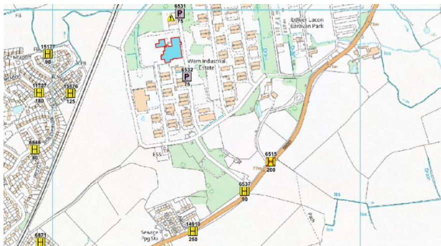
Figure 1 Fire hydrant map locations sent by Shropshire Fire and Rescue Service
