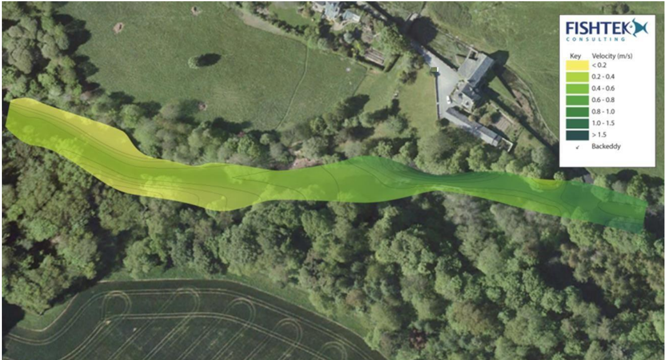
Figure 2.4. The velocity (m/s) of the downstream half of the PDR at approximately Q82 flow
