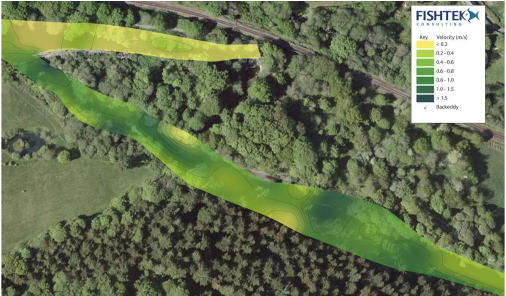
Figure 2.3. The velocity (m/s) of the upstream half of the PDR and the intake to the leat at approximately Q82 flow
