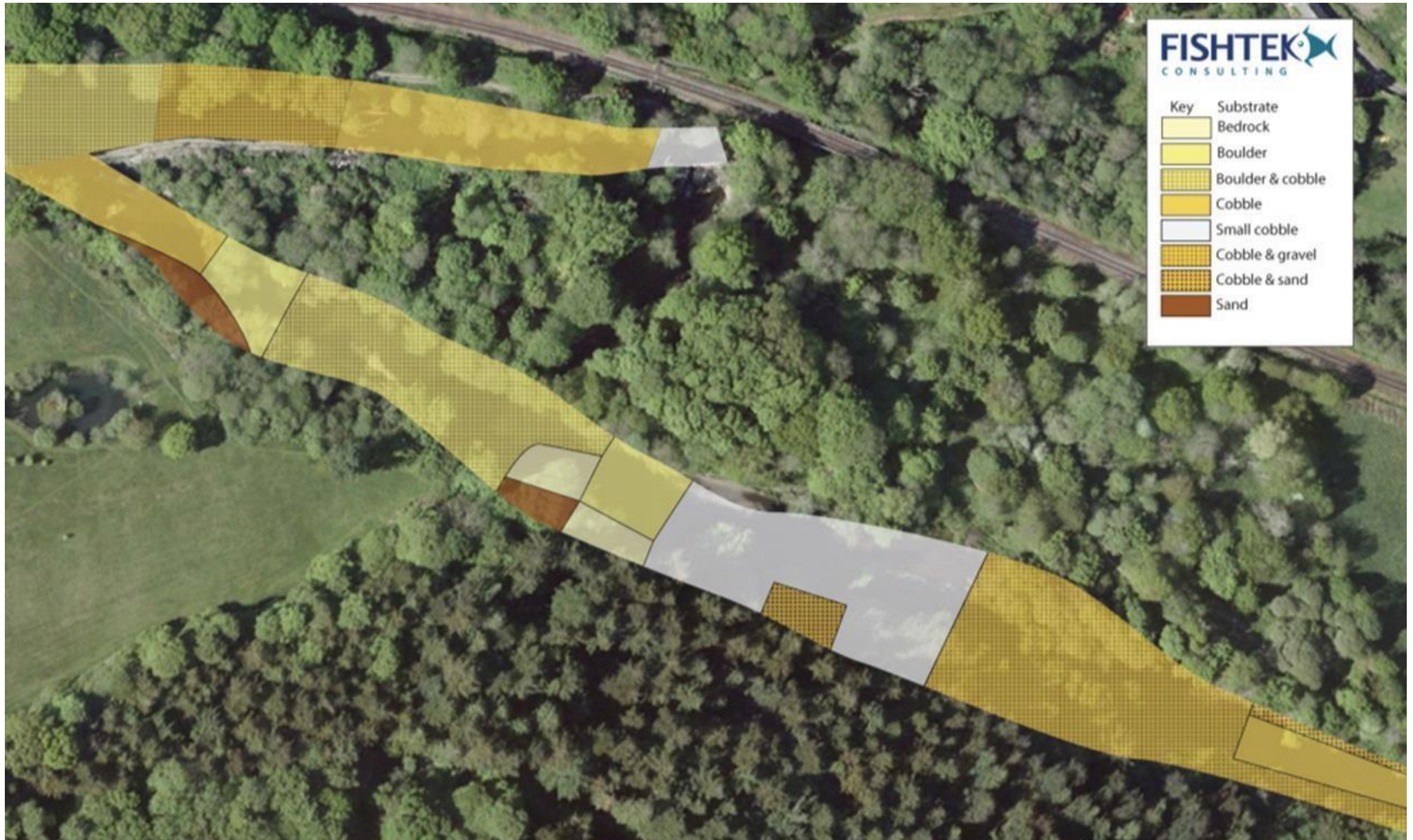
Figure 2.5. The predominant substrate composition of the upstream half of the PDR and the intake to the leat
