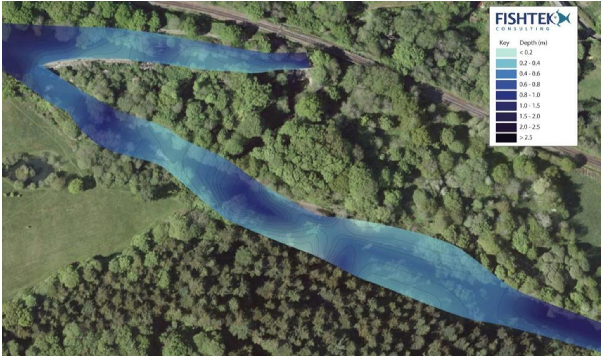
Figure 2.1. The depth (m) of the upstream half of the PDR and the intake to the leat at approximately Q82 flow
