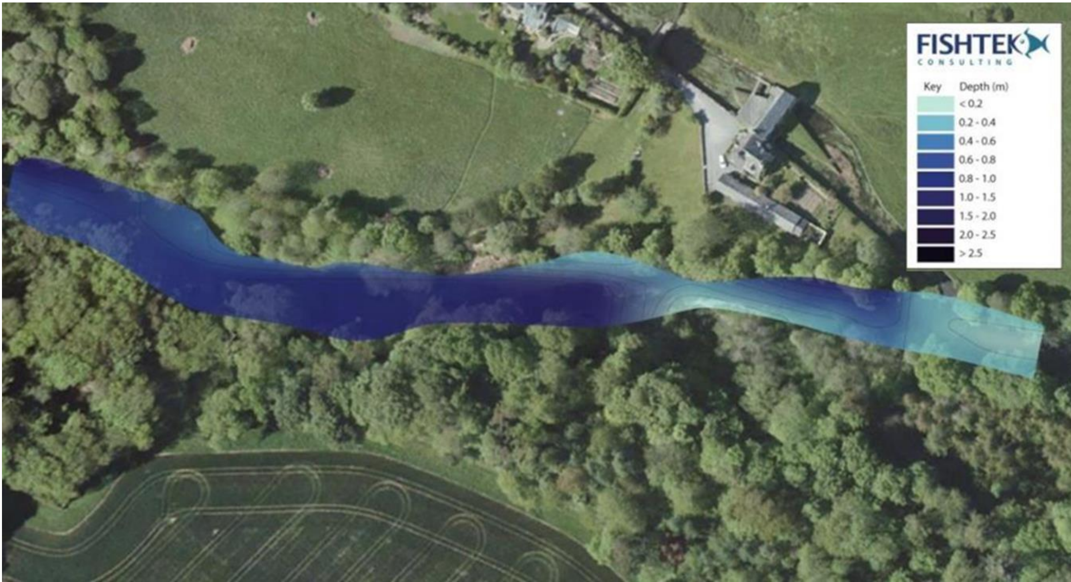
2Figure 2.2. The depth (m) of the downstream half of the PDR at approximately Q82 flow
