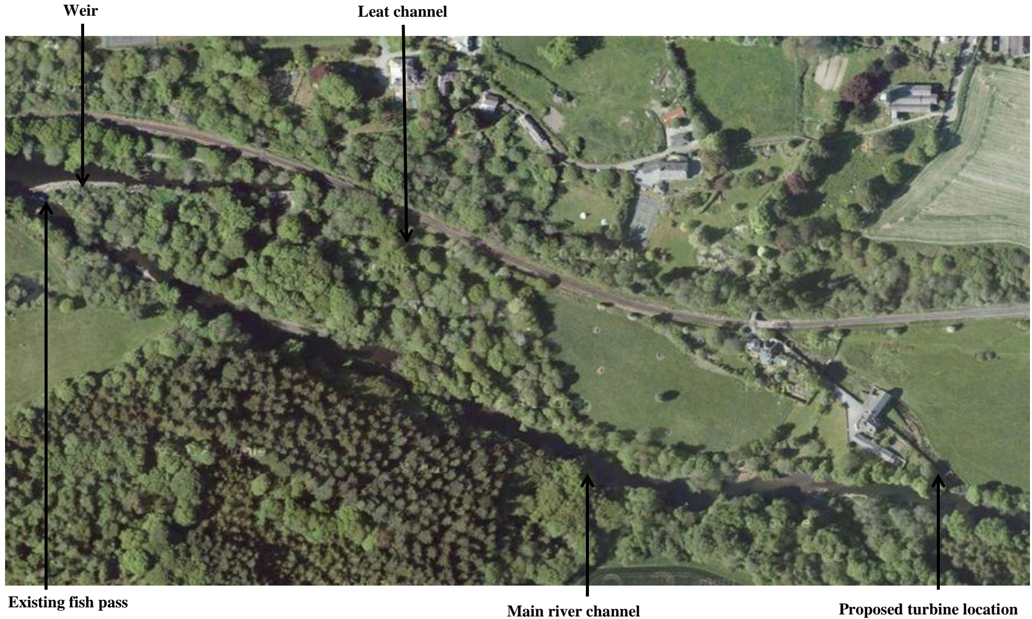
Figure 1. An aerial view of the site, showing the proposed turbine location in relation to the main river channel.
