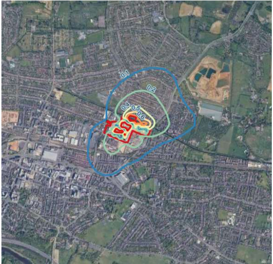
Figure 16 – Pollution Contour of NO 2 Annual Mean Concentrations during Worst Case – Cumulative Scenario
