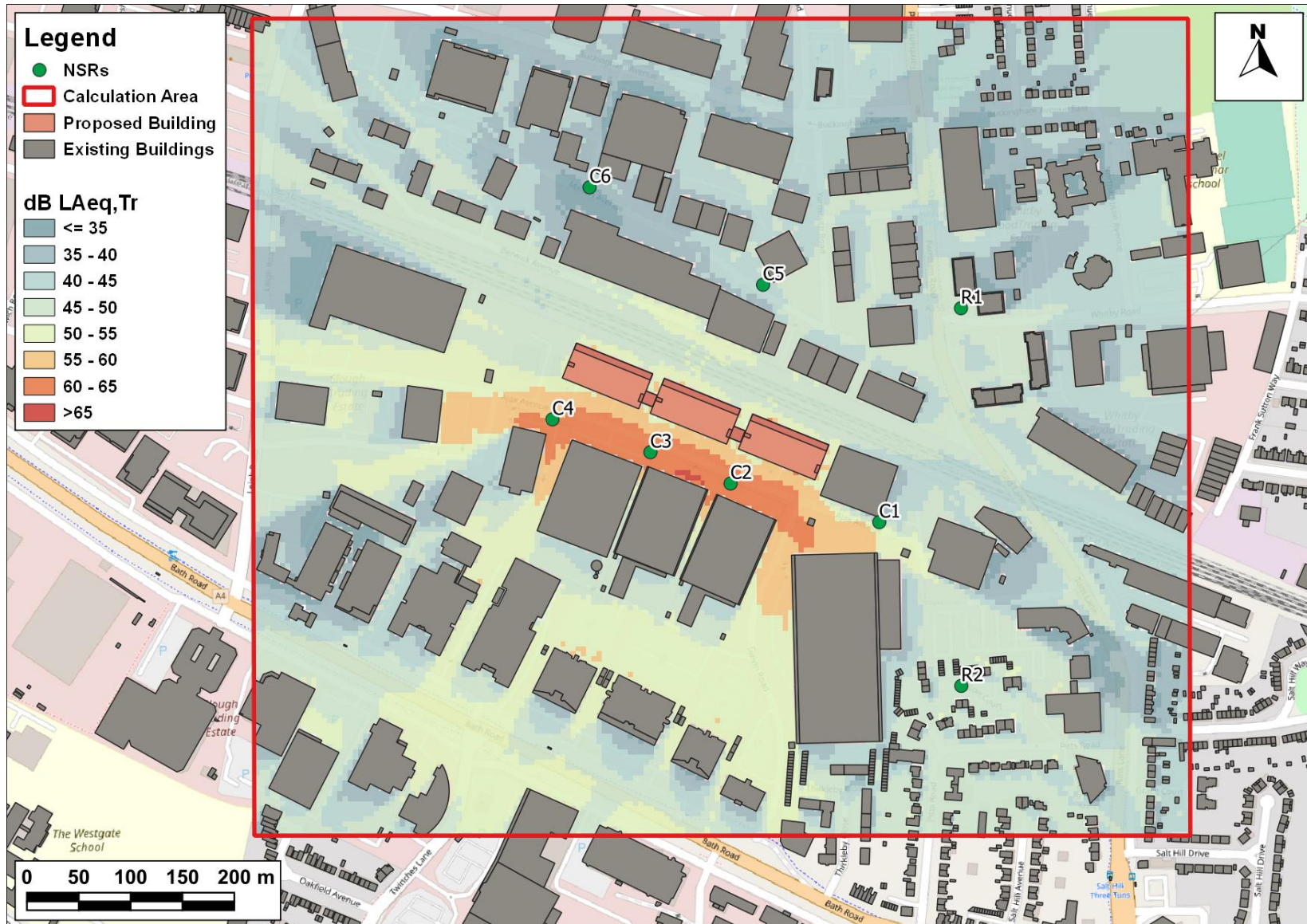
Figure A.4.1: Noise Map at 4 m – Chillers, DX Units, AHUs and Sound Break-out
