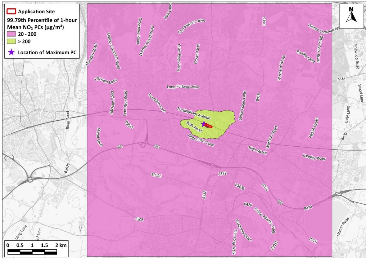
Figure 13: Contour Plot of the 99.79 th Percentile of Hourly Mean NO 2 PCs (Loss of Off-site Power Scenario)
