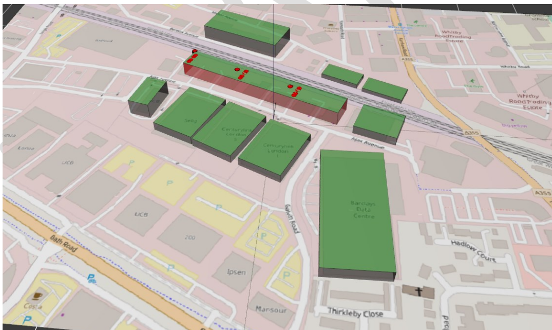
Figure A2.1: Modelled Generator Flue Outlet Layout (Red Circles) and Modelled Buildings (Green Rectangles)
