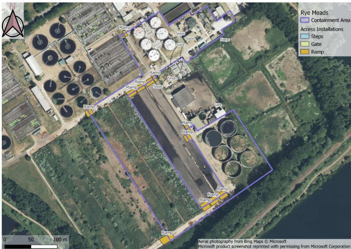
Figure 4-3 – O2 - 1 wide containment area - Old sludge drying beds as containment
