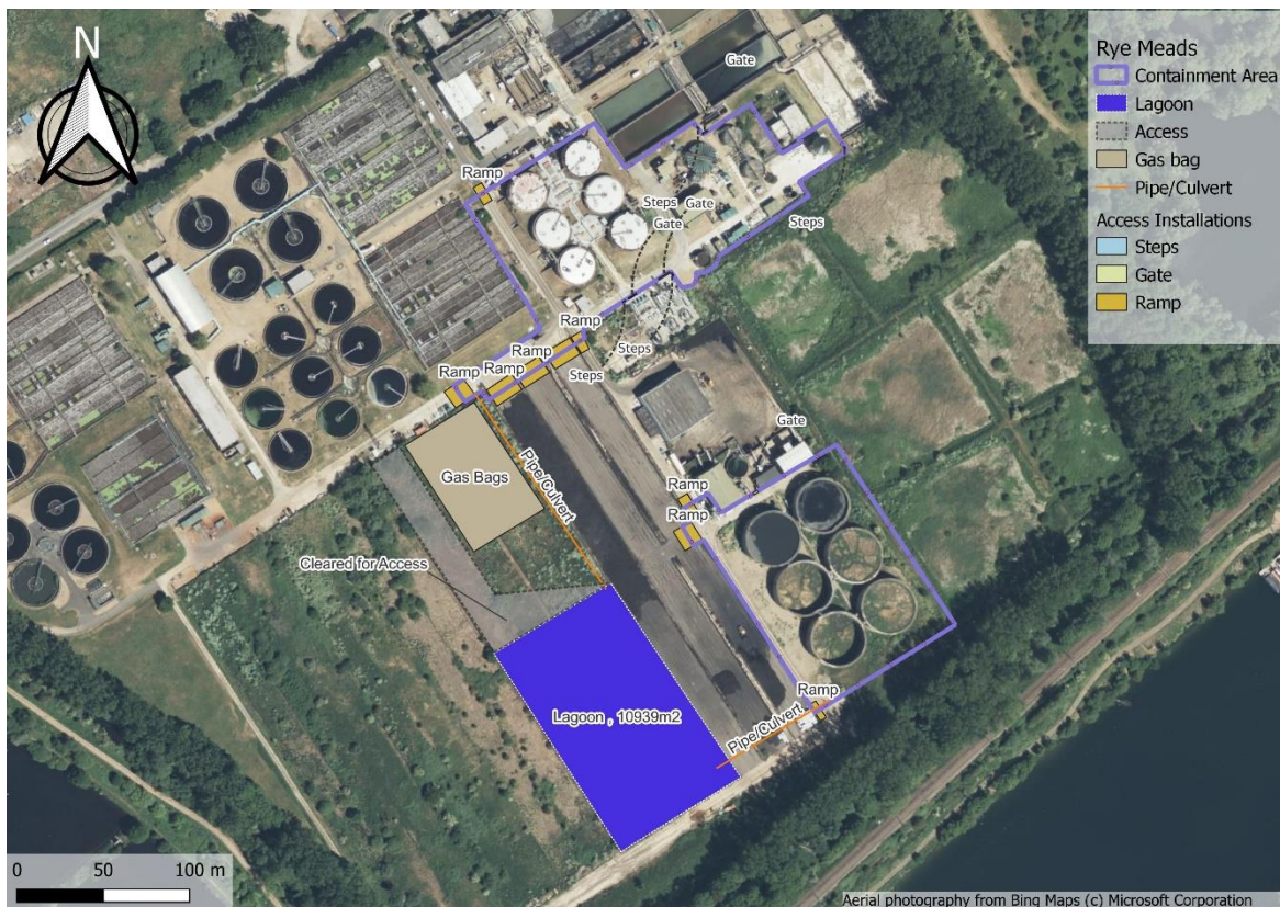
Figure 4-2 O1b - Lagoon Option – Gas bags on old sludge drying beds
