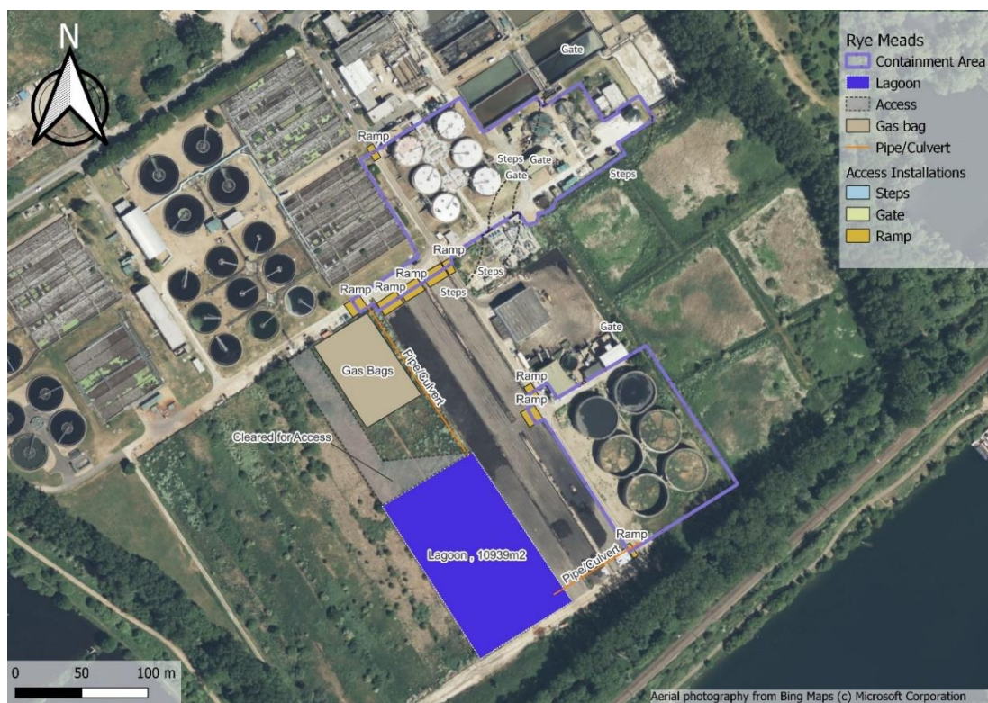
Figure 1-2 General layout of containment for Rye Meads STW where Gas bags over old sludge drying beds (Option 1b)
