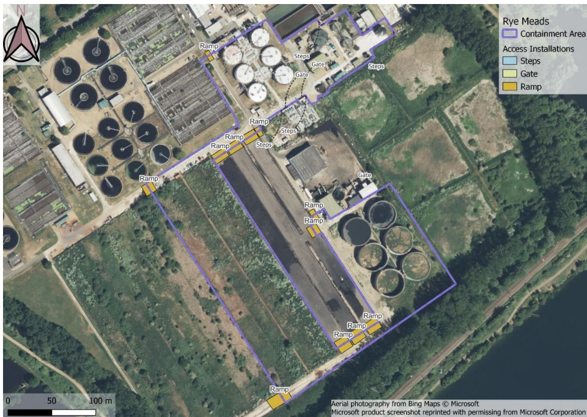
Figure 4-3 – O2 - single wide containment area with shallow storage on old drying beds
