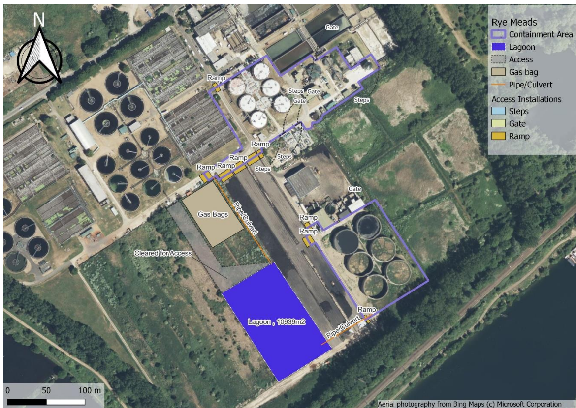
Figure 4-2 01b - Lagoon Option - If future gas bags on old sludge drying beds
