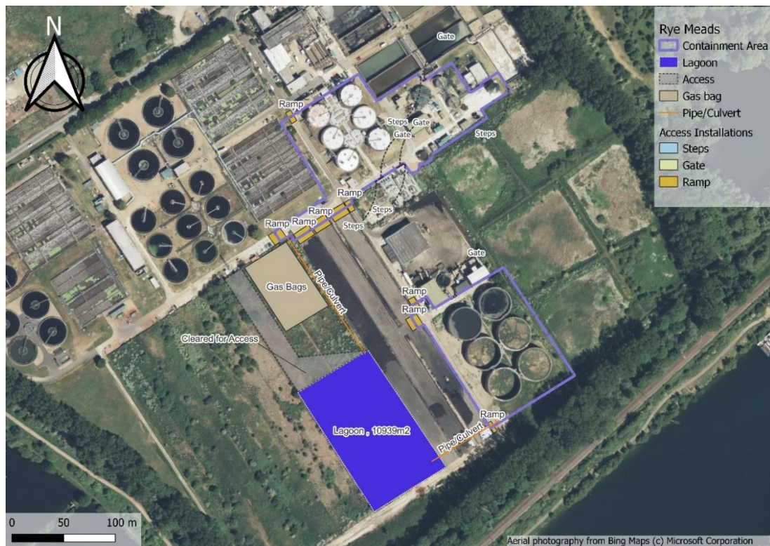
Figure 1-2 General layout of containment for Rye Meads STW if future gas bags on old sludge drying beds (Option 1b)
