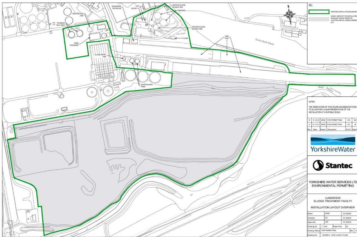
Fig 1 – Lundwood STF showing the installation boundary (green) and associated assets some of which may have the potential to cause bioaerosols
