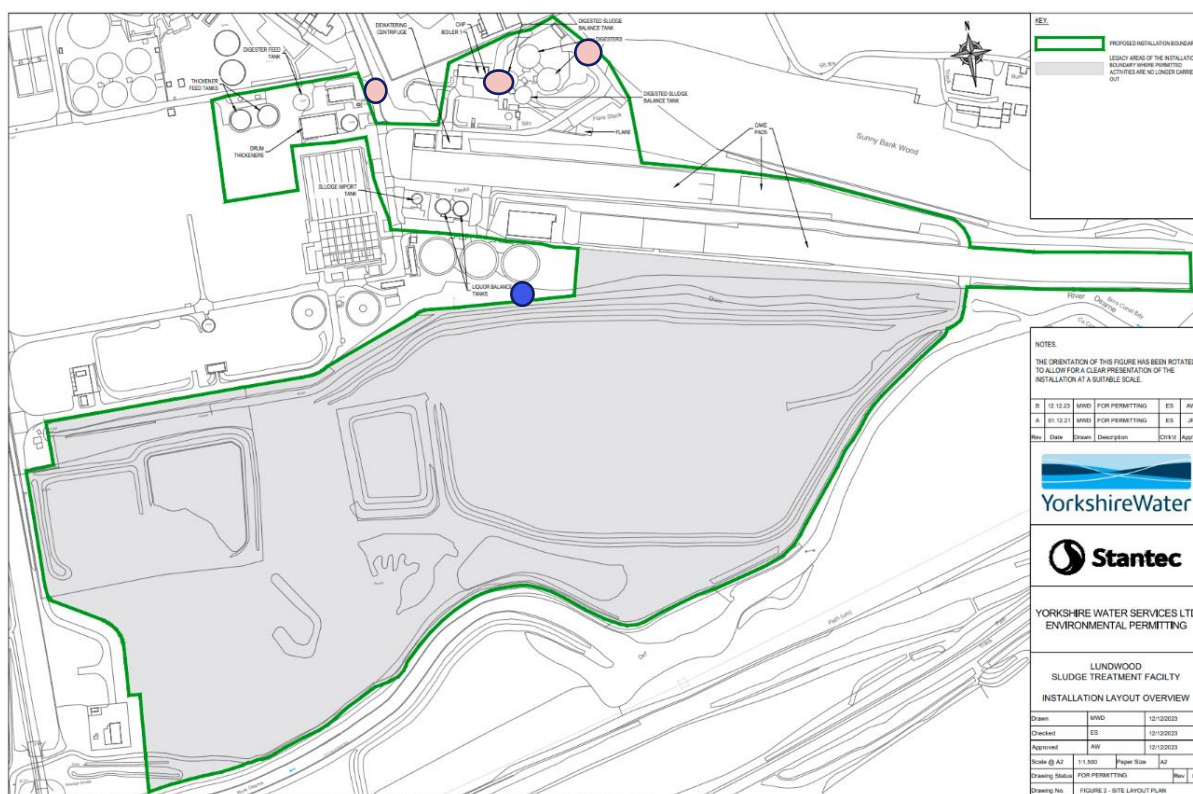
Figure 3 – Lundwood STF Site Plan showing the installation boundary (green) with bioaerosol monitoring locations marked (blue dot = upwind, pink dot = downwind)
