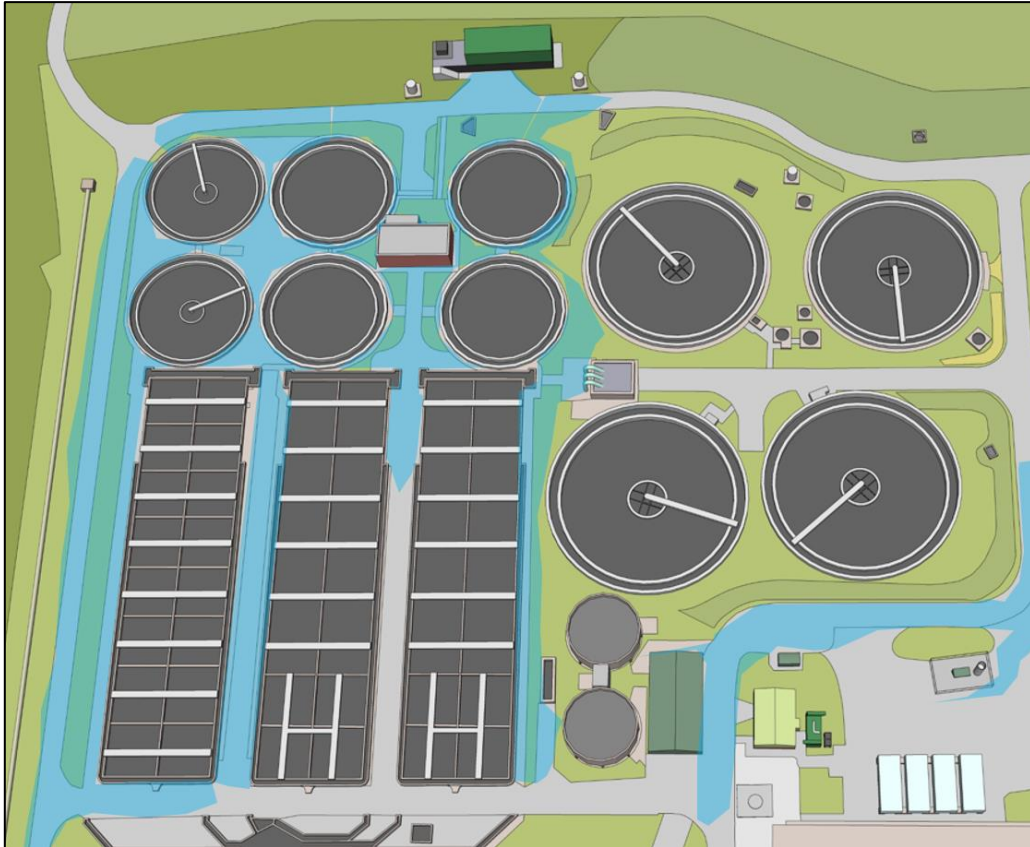
Figure 22. Spill pathway around the FST area.
