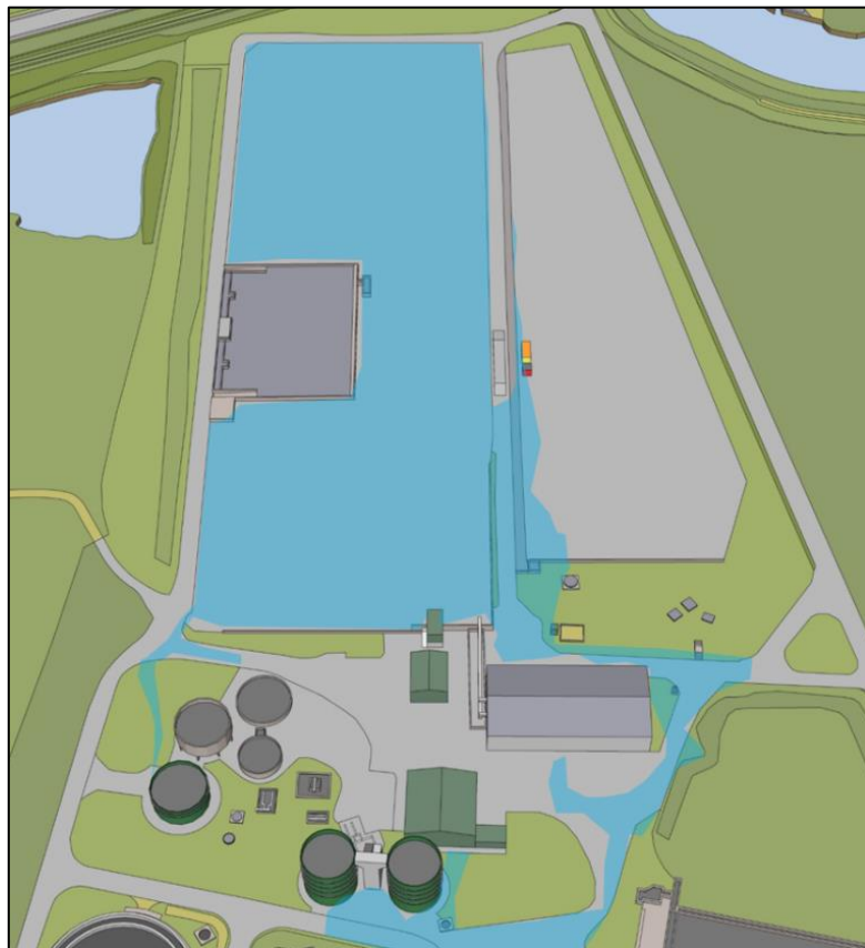
Figure 23. Spill pathway within and around the cake pads.
