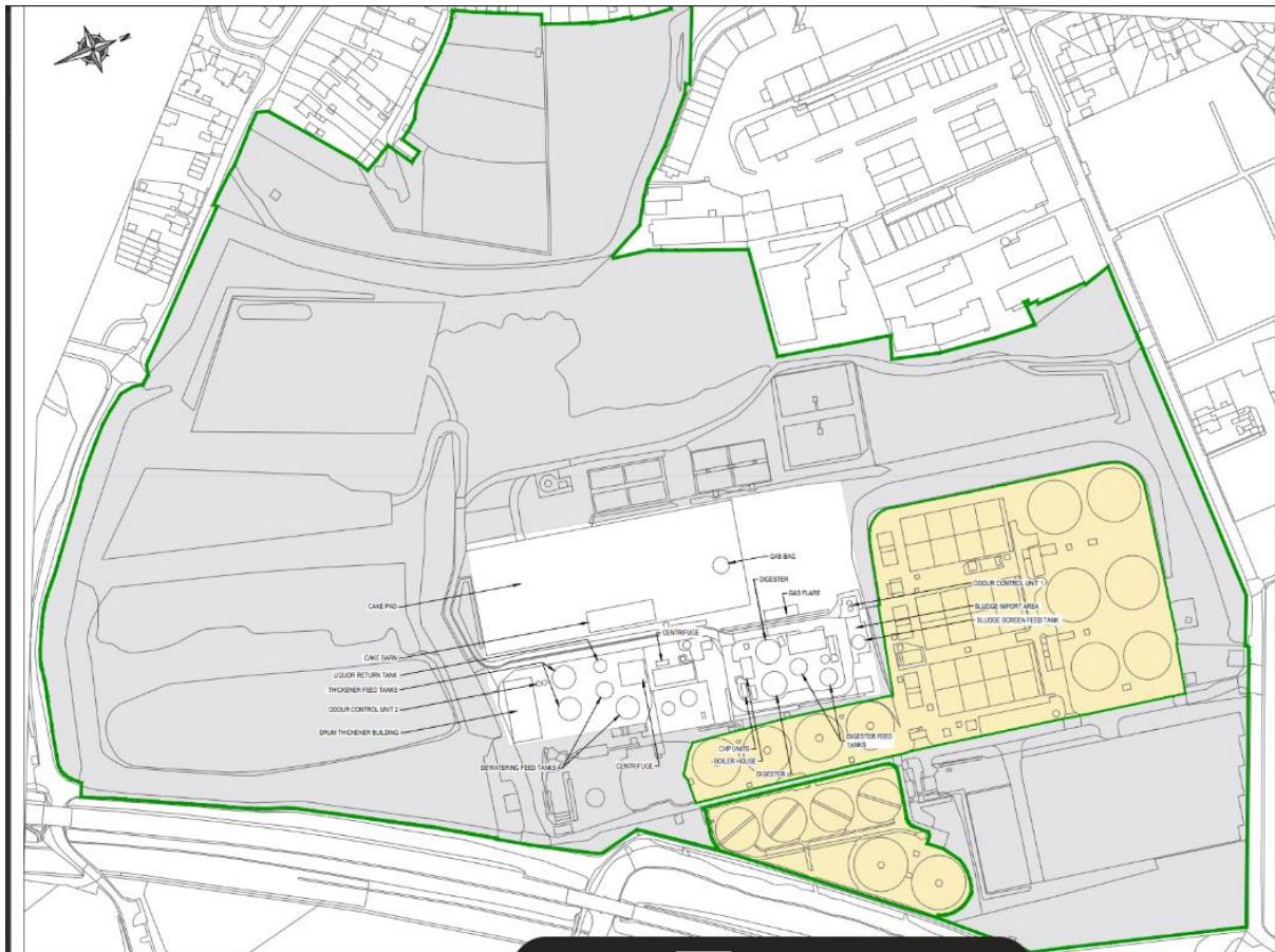
Fig 1 – Old Whittington STF showing the installation boundary (green) and associated assets some of which may have the potential to cause bioaerosols
