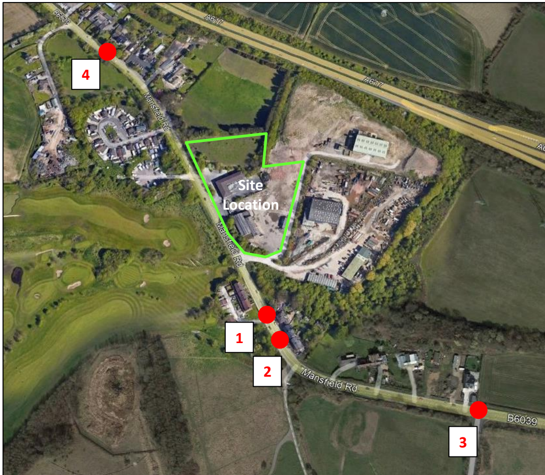
Figure 6 - Locations of Nearest Fire Hydrants
