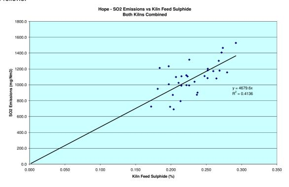
**CPI** Comments – the graph above demonstrates that there is a clear relationship between the kiln feed sulphide content and the stack  $SO_2$  emissions. Typically an increase of 0.1% kiln feed sulphide would be expected to increase the stack  $SO_2$  by approximately 468 mg/Nm<sup>3</sup>.
