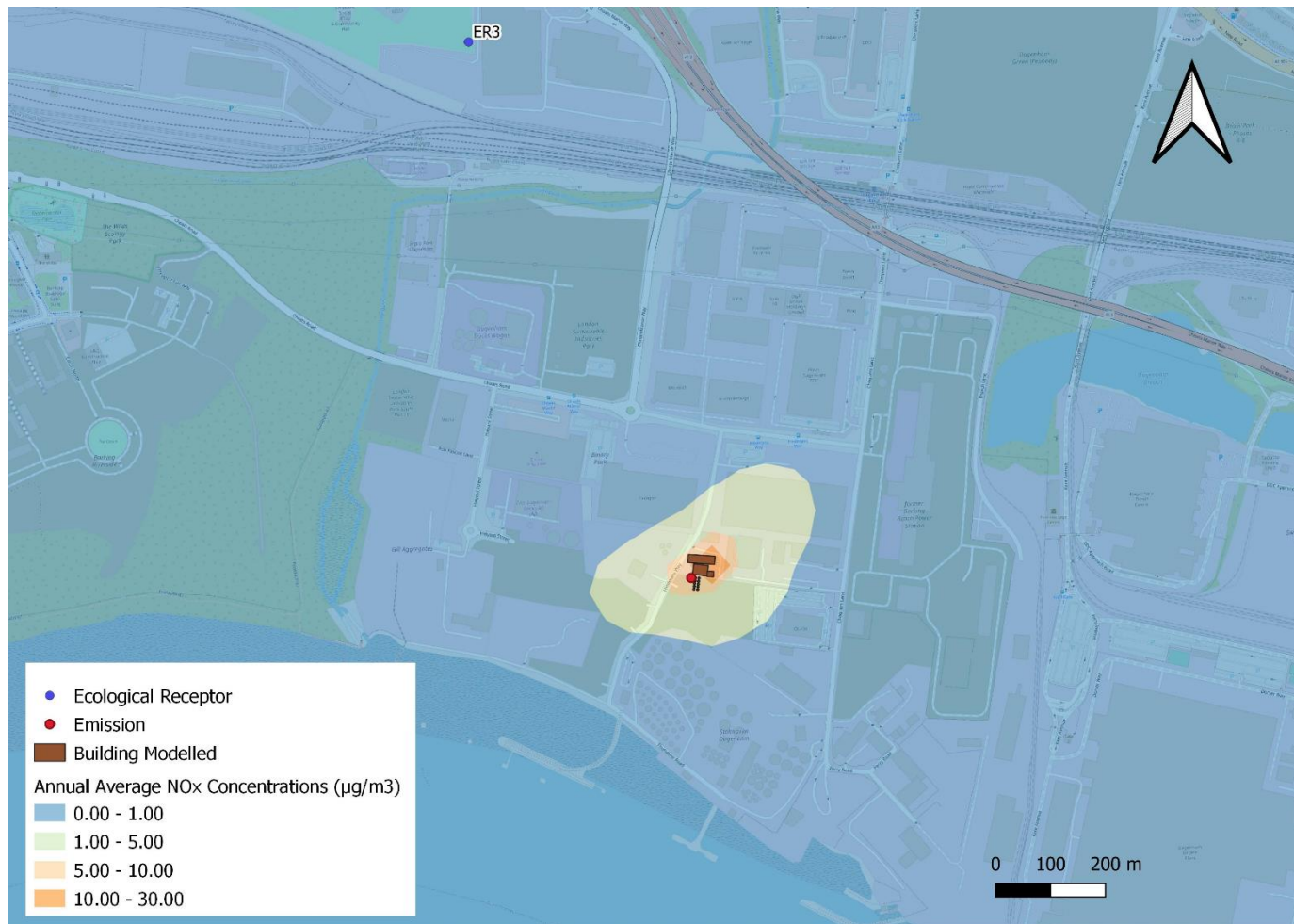
Figure C3: Predicted Annual Average NO x Concentrations (µg/m 3 ) PEC – relevant for ecological receptor locations – 2022 met data
