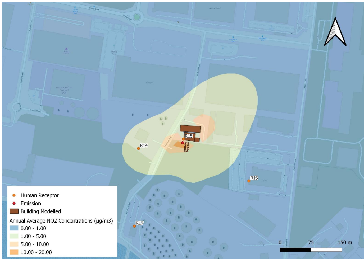
Figure C1 Predicted Annual Average NO 2 Concentrations (µg/m 3 ) PEC – relevant for human receptor locations – 2022 met data
