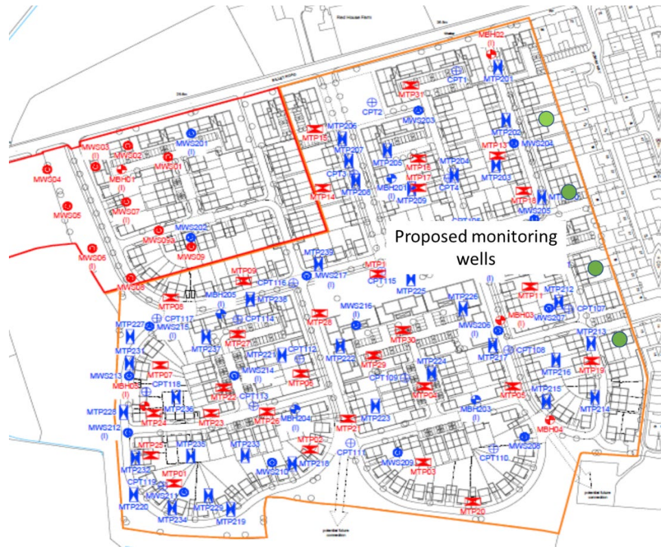
Figure 3: Ground gas monitoring locations during filling.
