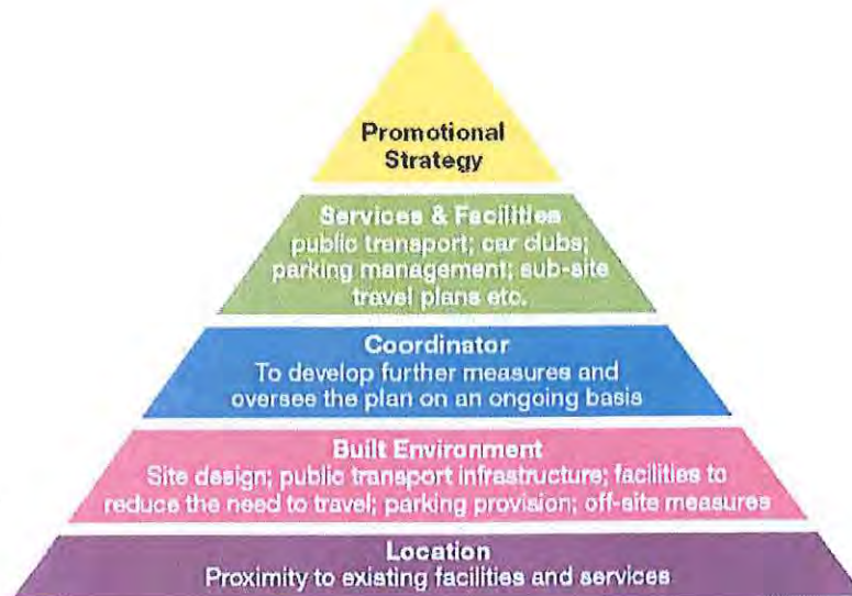
Figure 2 – Travel Plan Pyramid ('Making Residential Travel Plans Work' DfT 2007)
