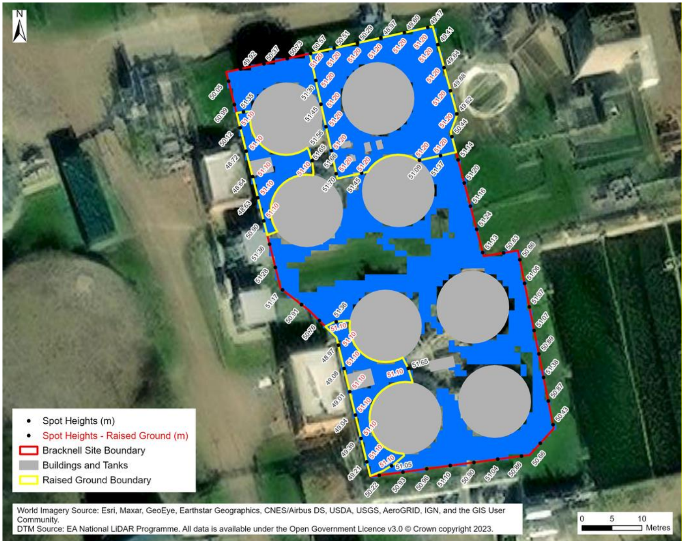
Figure 14: Area 3A Spot Levels along Containment Boundary
