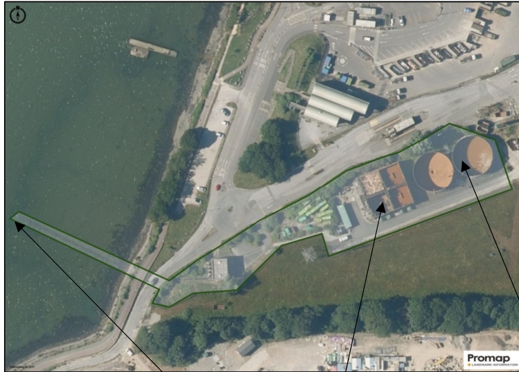
Plate 1.1: Aerial view (2017) showing entire Chelson Meadow LTP permit boundary in green, with the outfall to the River Plym, four Sequential Batch Reactors (SBRs) and two storage tanks.
