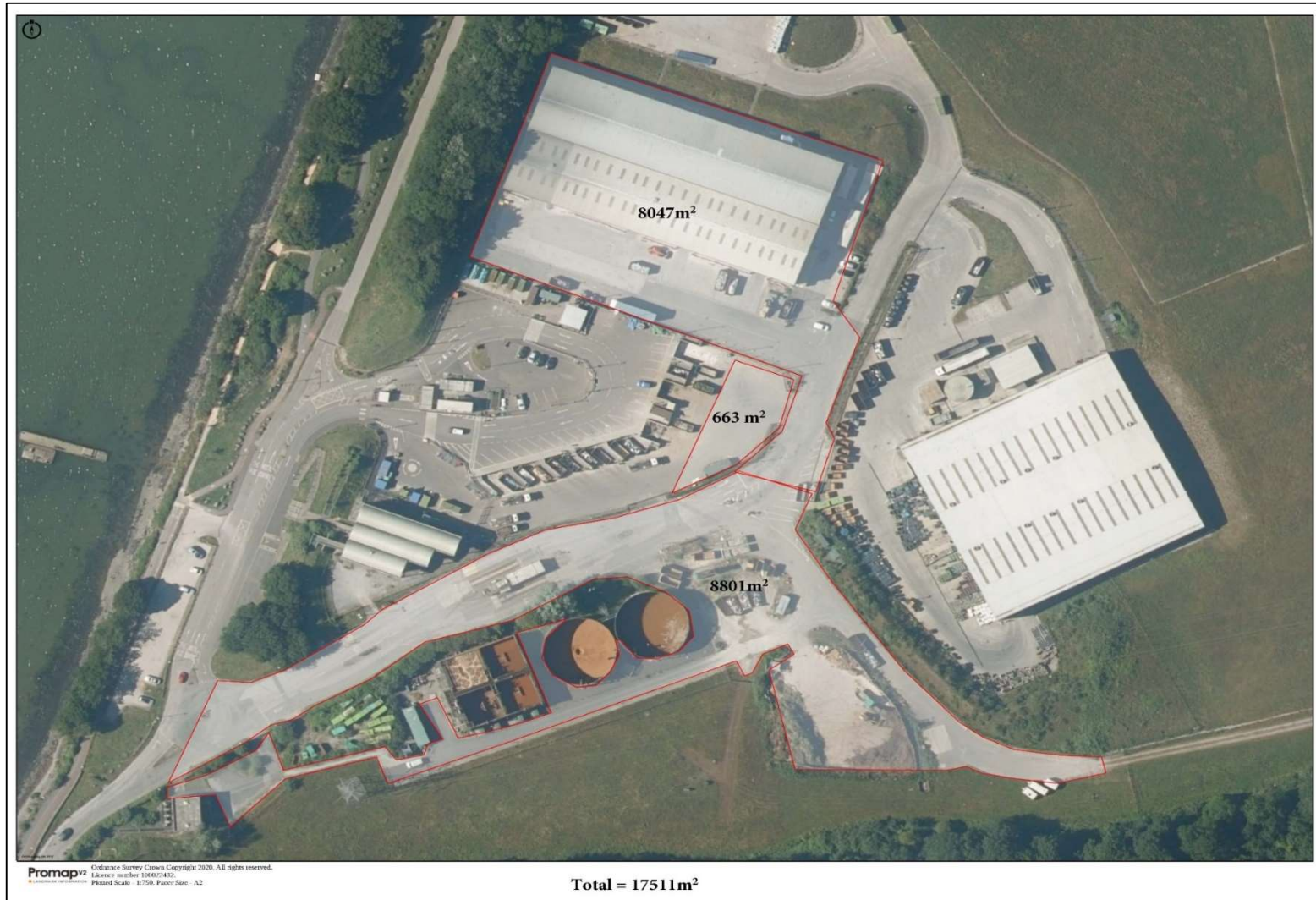
Plate 2.5: Aerial view focussing on the section hatched in green on Figure 2.5 and quantifying three key areas of impermeable surface draining to the LTP.
