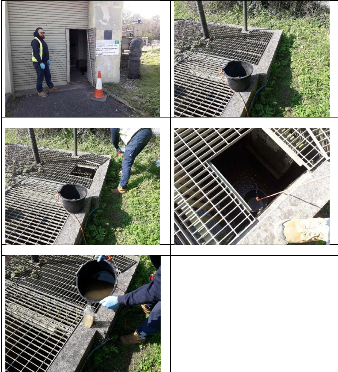
Plate 10: Step-by-step procedure for obtaining a sample of treated leachate from the outfall during discharge at high tide
