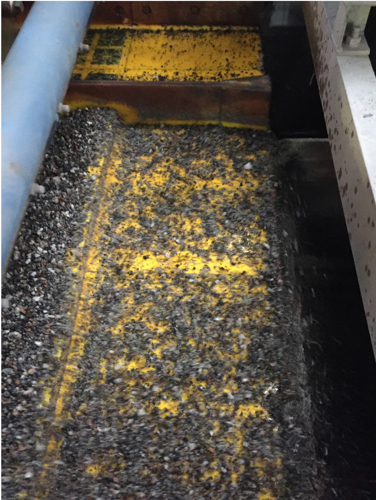
Figure 2: Example of Secondary DMS Screen
