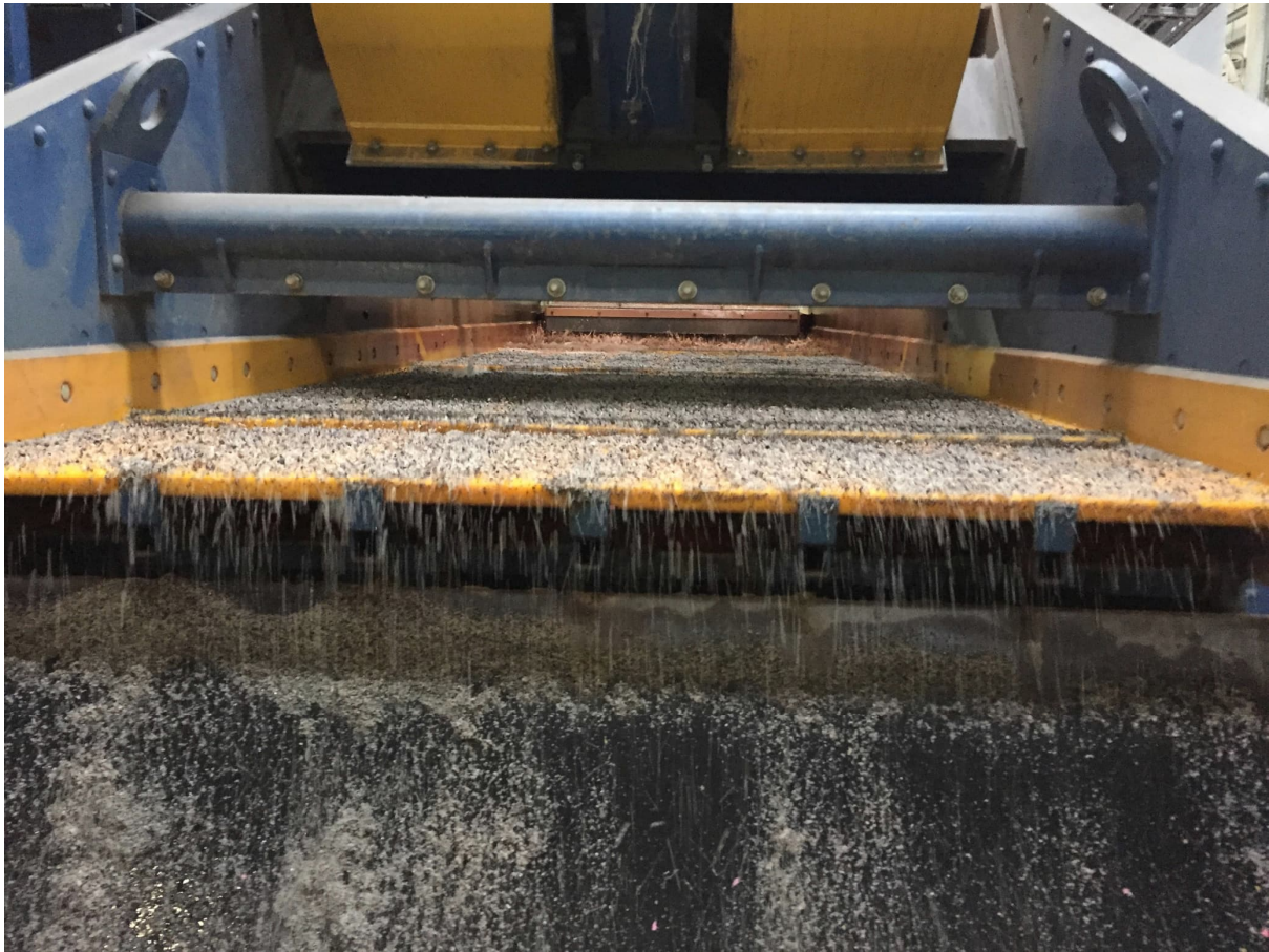
Figure 1: Example Wet Screen with 0.8mm Deck
