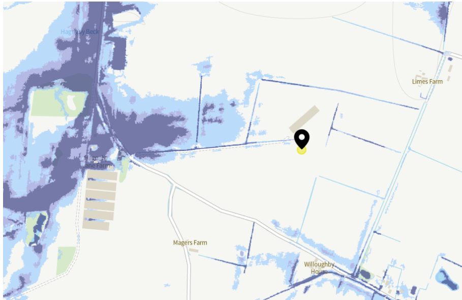
Surface water flood risk map identifying proposed unit location in low risk land. Medium to high risk is identified in light and dark blue respectively.
