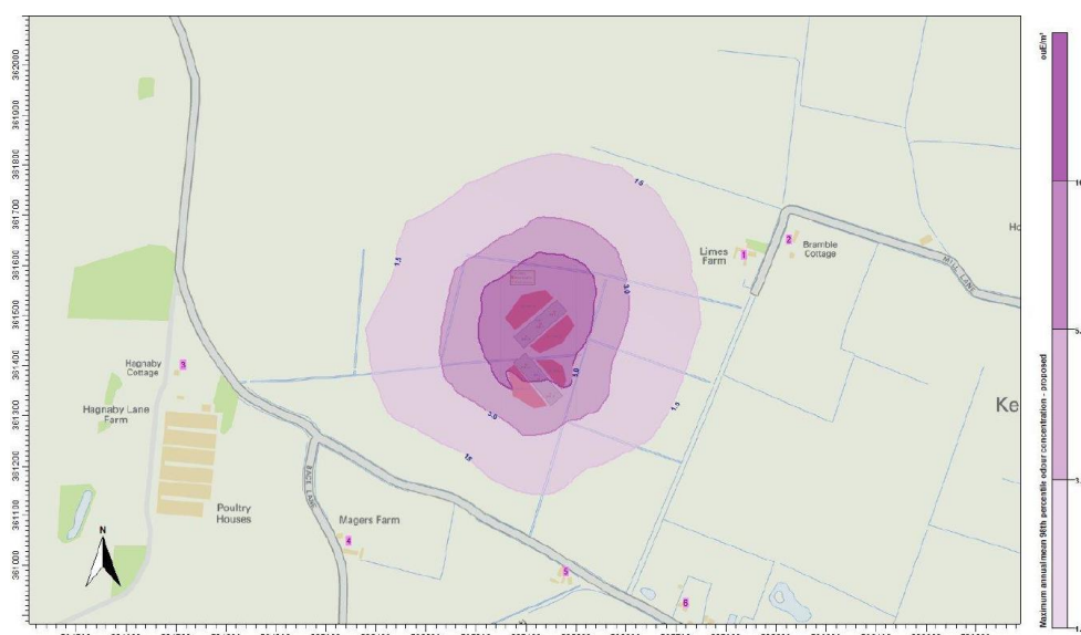
Figure 7 Extract: Predicted maximum annual 98th percentile hourly mean odour concentration in area surrounding poultry unit.
