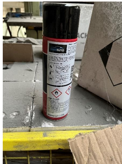
Flammable products stored on mezz.
