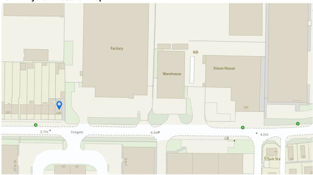
All 3 hydrants indicated (green dots) are on the same 150mm main. A hydrant of this size will deliver on average 1500 Litres per minute at 3 bar pressure. This would be dependent on the time of day and the
