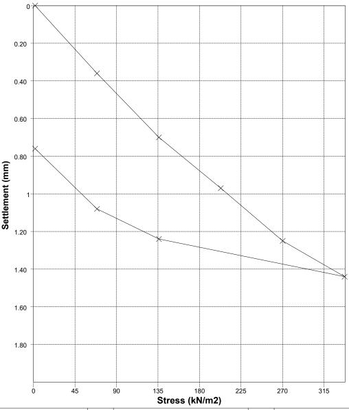
Max applied pressure (kN/m²) 337.35 Stress at 1.25mm plate settlement (kN/m²) 270.22 Max deformation (mm) 1.44
