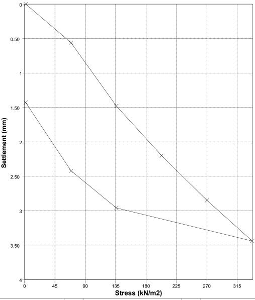
Max applied pressure (kN/m²) 337.35 Stress at 1.25mm plate settlement (kN/m²) 119.24 Max deformation (mm) 3.44
