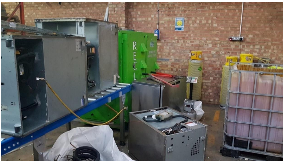
Figure 1. Refrigerant and oil recovery system
