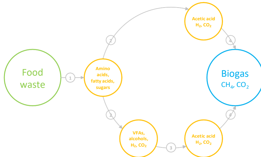
Figure 6 Schematic of the AD process steps; (1) hydrolysis (2) acidogenesis (3) acetogenesis (4) methanogenesis
