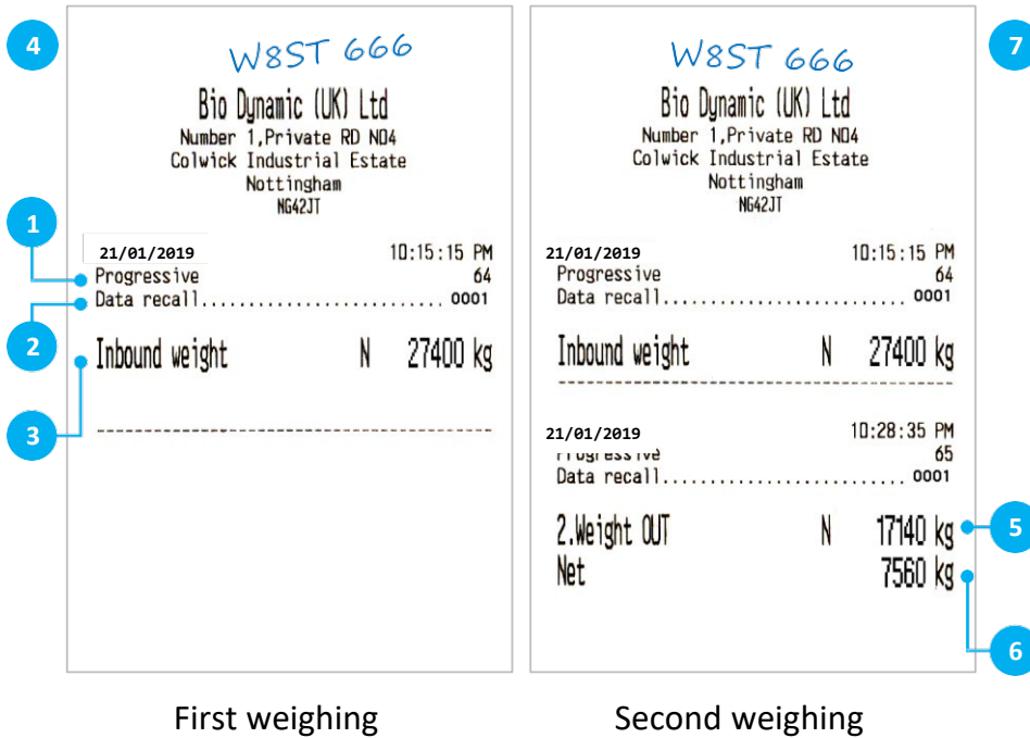
Figure 1 Examples of weighbridge tickets for incoming (first weighing) and outgoing (second weighing) waste vehicles. (1) The number of times the weighbridge has been used so far, (2) the weighbridge ticket number for the current waste transfer, (3) the vehicle gross weight, (4) the vehicle registration number, (5) the vehicle tare weight, (6) the waste delivery net weight, (7) the vehicle registration number
