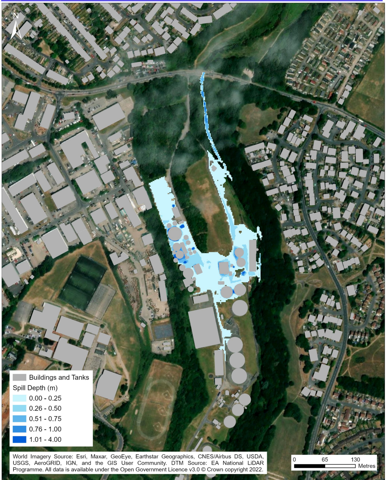
Figure 2.2 Uncontrolled spill of Mansfield Sewage Treatment Works
