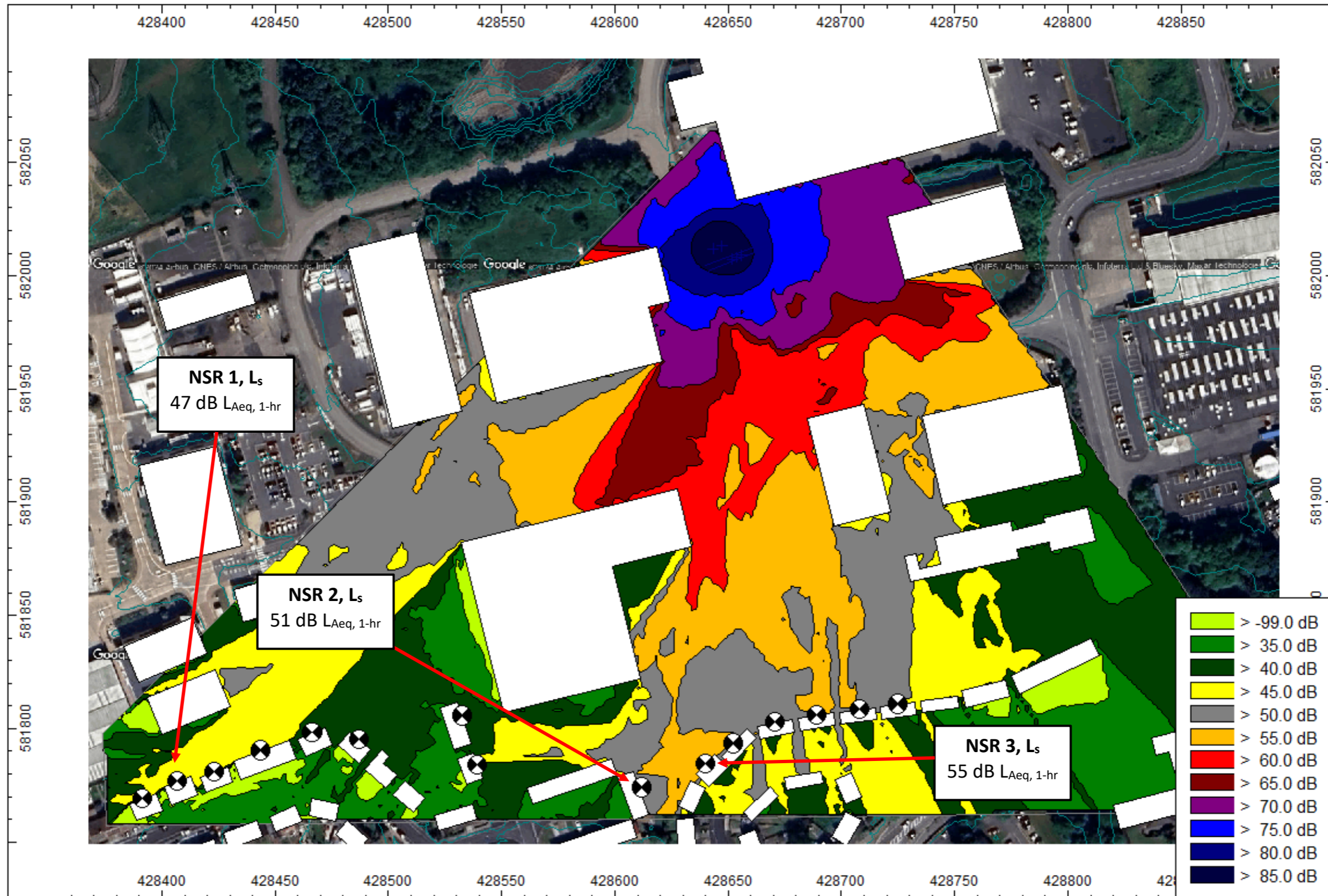
Figure 7: Sound contours at 1.5 m (ground floor window height), showing the predicted specific sound level, L_{Aeq,1hr} based on current operation
