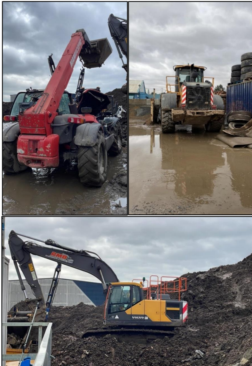
Figure 2: Heavy Plant machinery (Manitou Telehandler, Bell Loading Shovel, and Volvo EC220 Excavator) on site.
