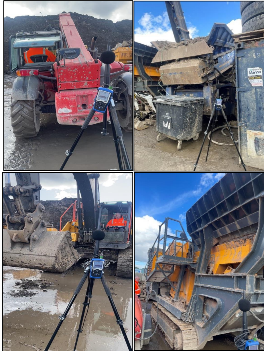
Figure 5: Pictures showing plant source measurements in progress
